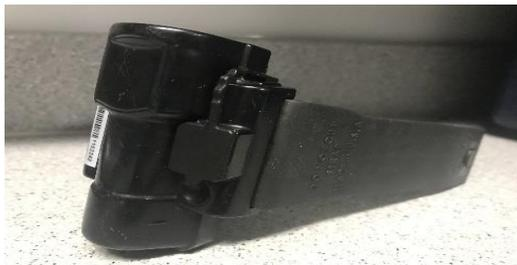
TAD/ Transdermal Alcohol Detector transmitter
