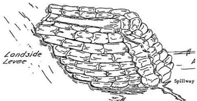
Figure 11 - Sketch of a ring levee tied to a levee slope, with spillway.
