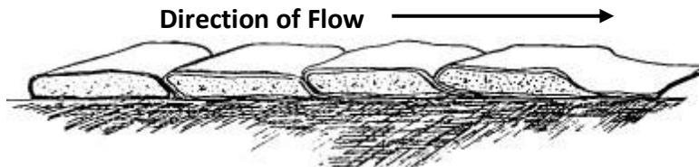
**Figure 3 – Overlap sandbags lengthwise and parallel to river flow.**
