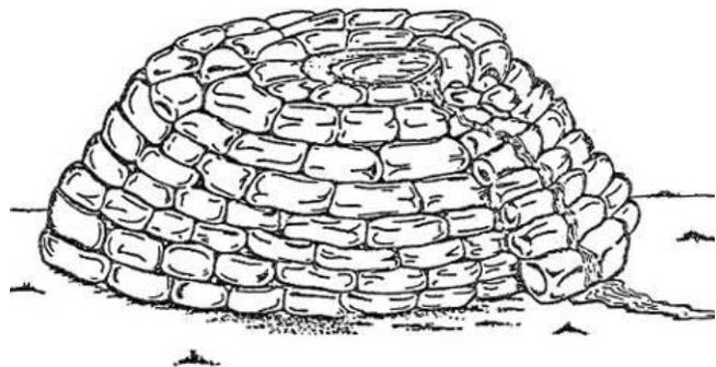
Figure 10 - Sketch of a typical ring levee with spillway.
