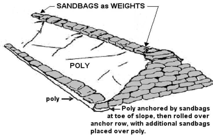
**Figure 5 – Preferred method of tucking under and anchoring poly with two rows of sandbags.**
