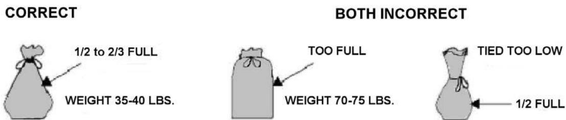
Figure 1 – Correct and incorrect sandbag preparation.
