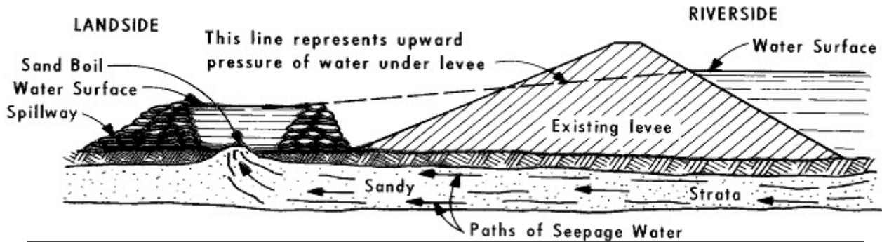
Figure 9 - To treat the sandboil, the pressure of the seepage water is counterbalanced by hydrostatic pressure from the column of water in the ring levee.
